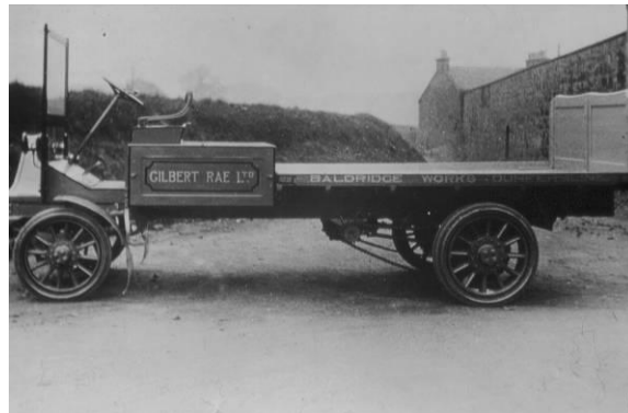
Gilbert Rae's Edison Electric Lorry – The boxed area behind the driver housed a series of batteries which required charging each night.
